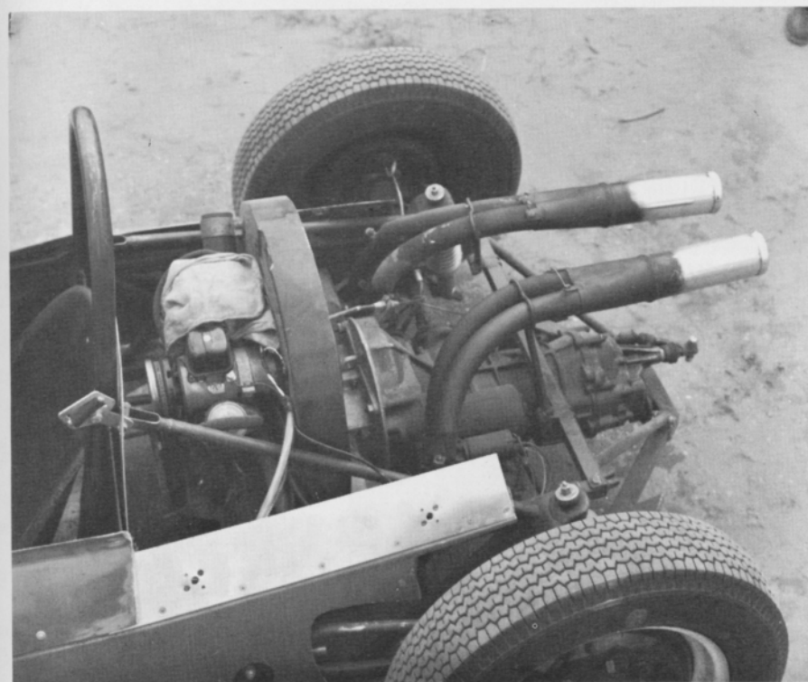
The engine is placed forward and the transmission rearward, a la Porsche Spyder.
